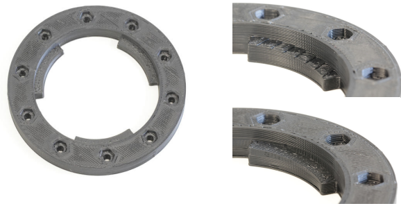
Fig. 7. Example for adaptive slicing. Bayonet coupling (left) and close-ups of the bayonet printed with static (top right) and adaptive (bottom right) resolution. In this application, the grade-smoothness is crucial for the function, while the optical surface quality is less important. The steps generated by non-minimal layer height will prevent the inner and outer parts from gliding into the lock-position. Note that automatic adaptive slicing generates thin layers only where required, while maximal layer height h_{\text{max}} is used for the vertical structures below and above the actual bayonet part to improve printing speed.
